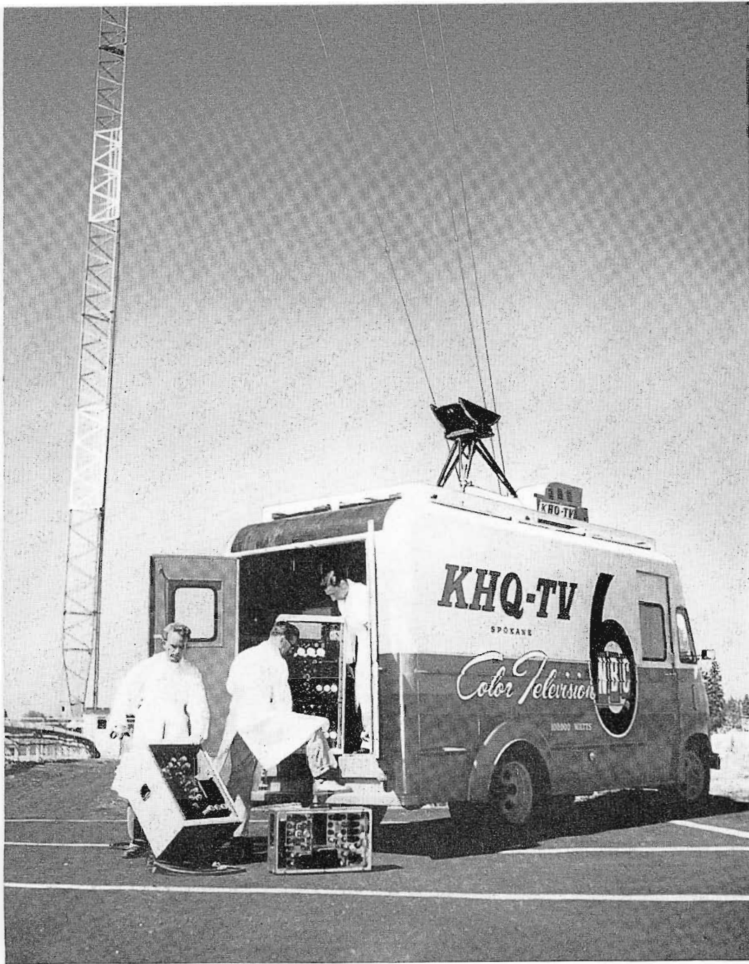
FIG. 17. Rack equipment for KHQ-TV color remote truck is built into small portable units. These are used both in the truck and in the studio.
