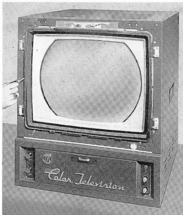
FIG. 5. Decorative bezel surrounding picture area is removed for access to the equalizing magnets and safety glass.
